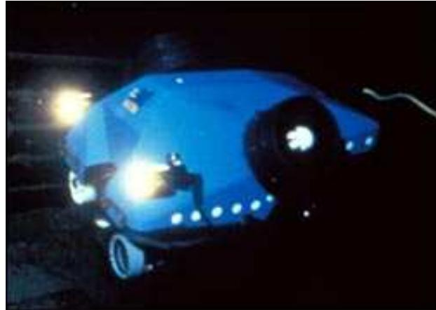
Remotely piloting a submersible requires a full attitude sensor. Heading data is necessary to navigate the vehicle to its destination. Pitch and roll data is also required to provide an accurate picture of the vehicle's orientation. Other important features of the sensor package are wide bandwidth, low power consumption, and high reliability.
