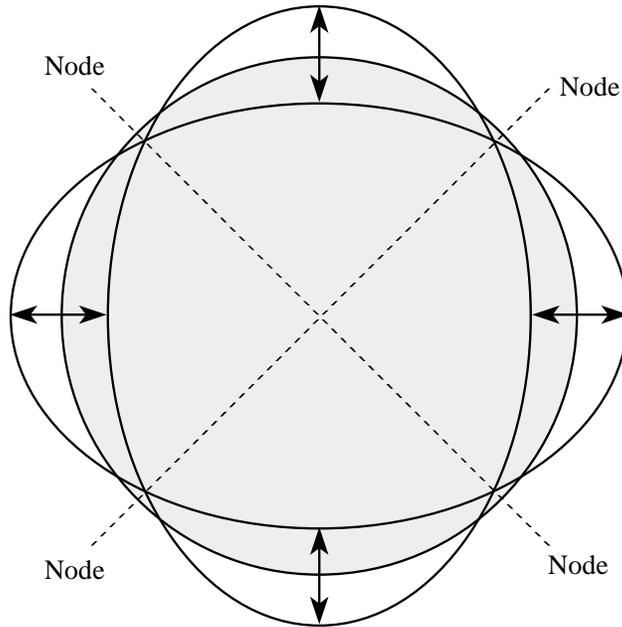
**Figure 1. Gyro vibration pattern.**
