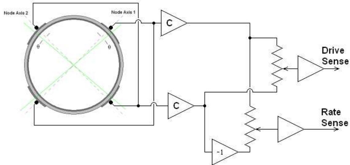
**Figure 14. Skew sensing circuitry**
