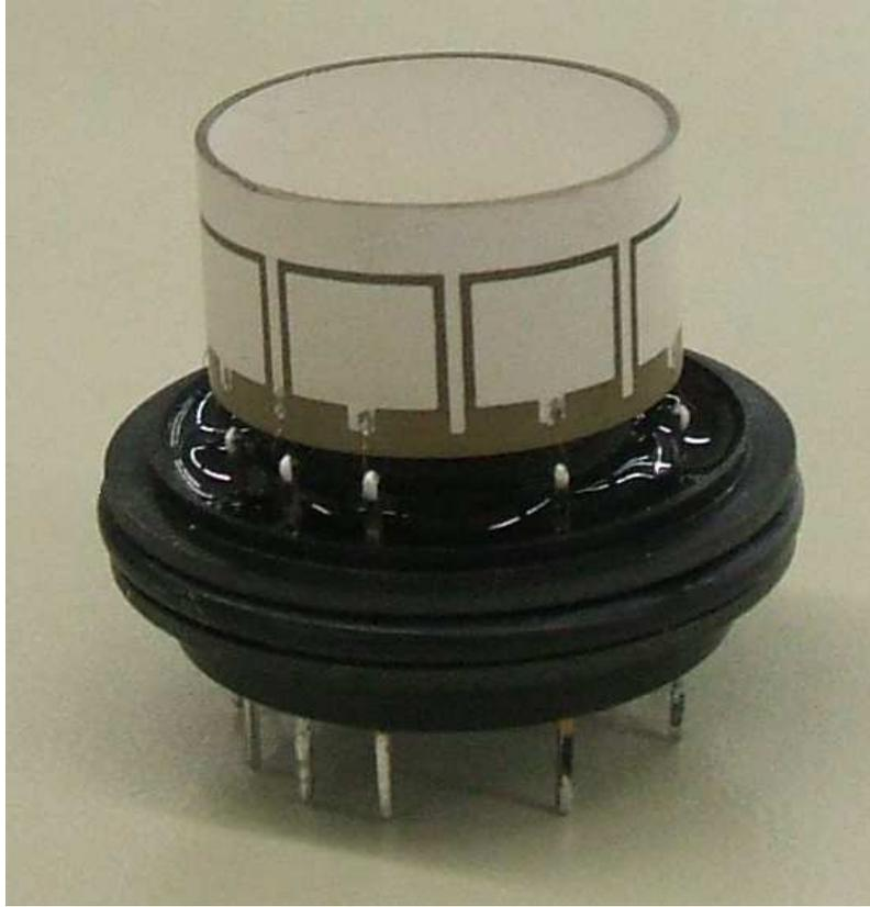
**Figure 2. The piezoceramic cup gyro.**
