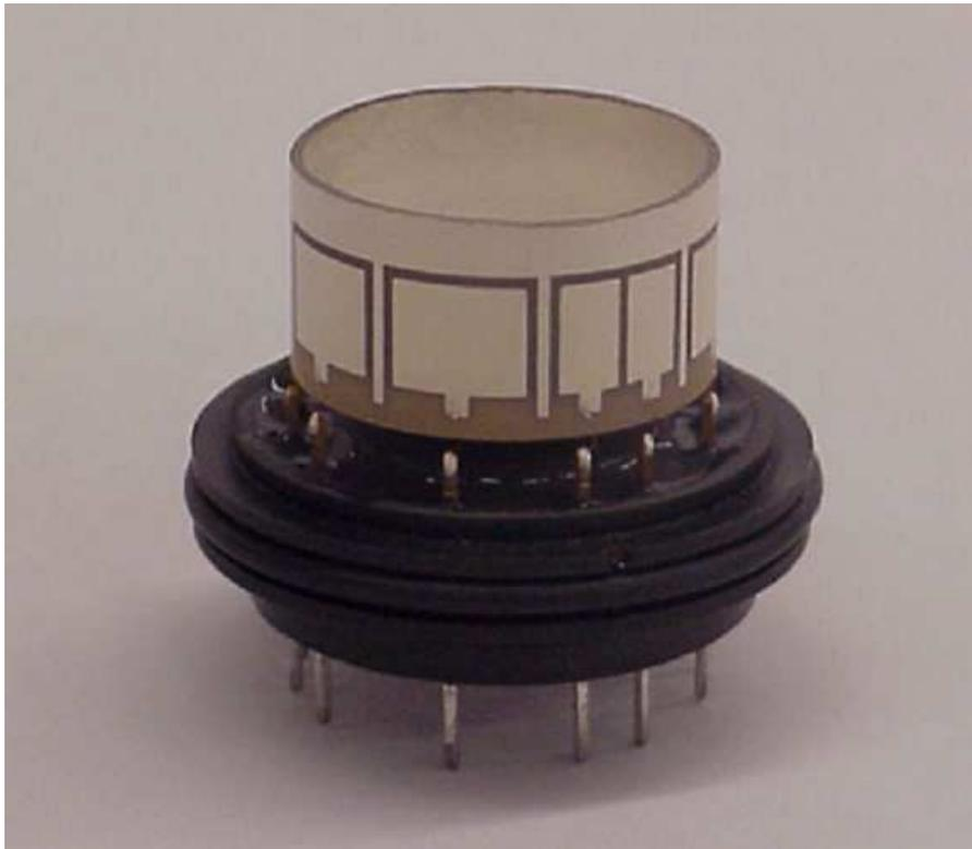
**Figure 4. Gyro split electrode.**
