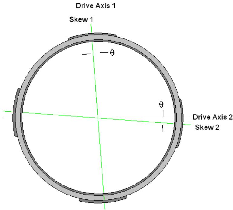
**Figure 15. Skewed Drive Electrodes.**
