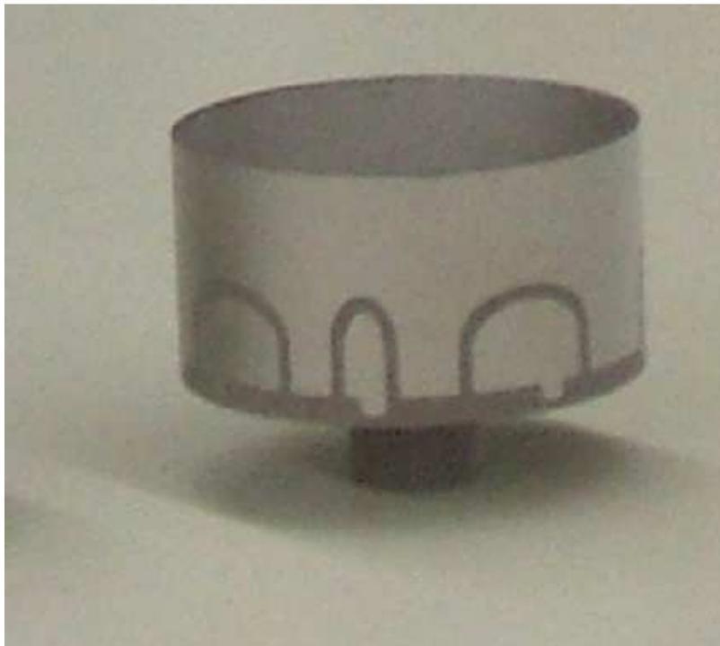
**Figure 17. Skew electrode pattern**
