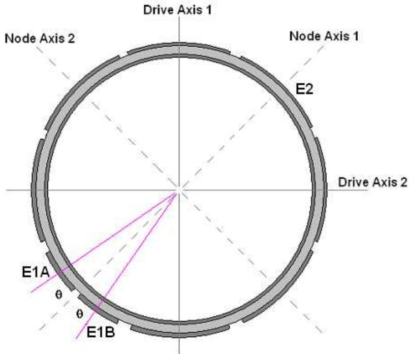
**Figure 9. Gyro split electrode in the sense position.**
