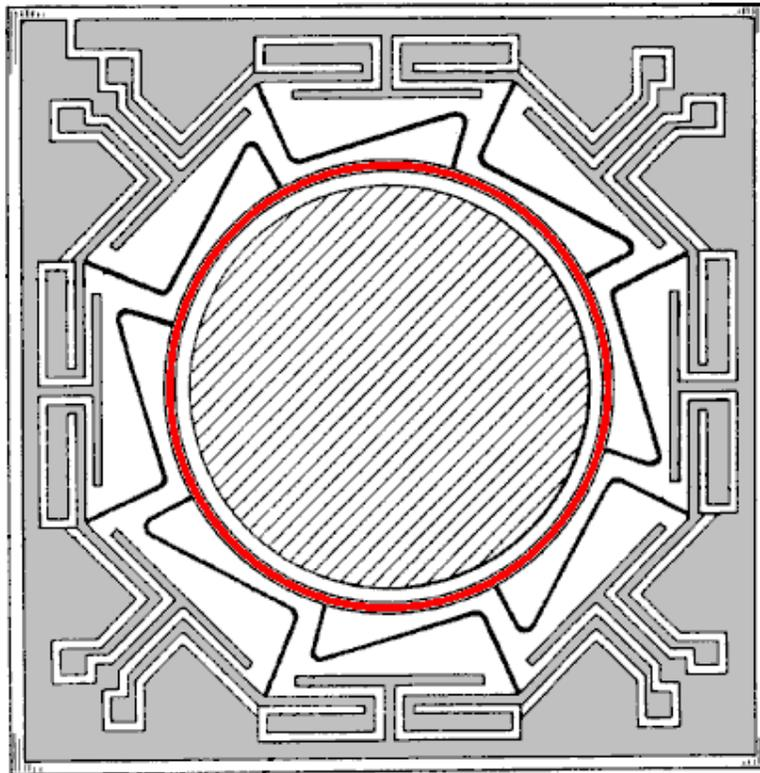
**Figure 20. Ring gyro configuration**
