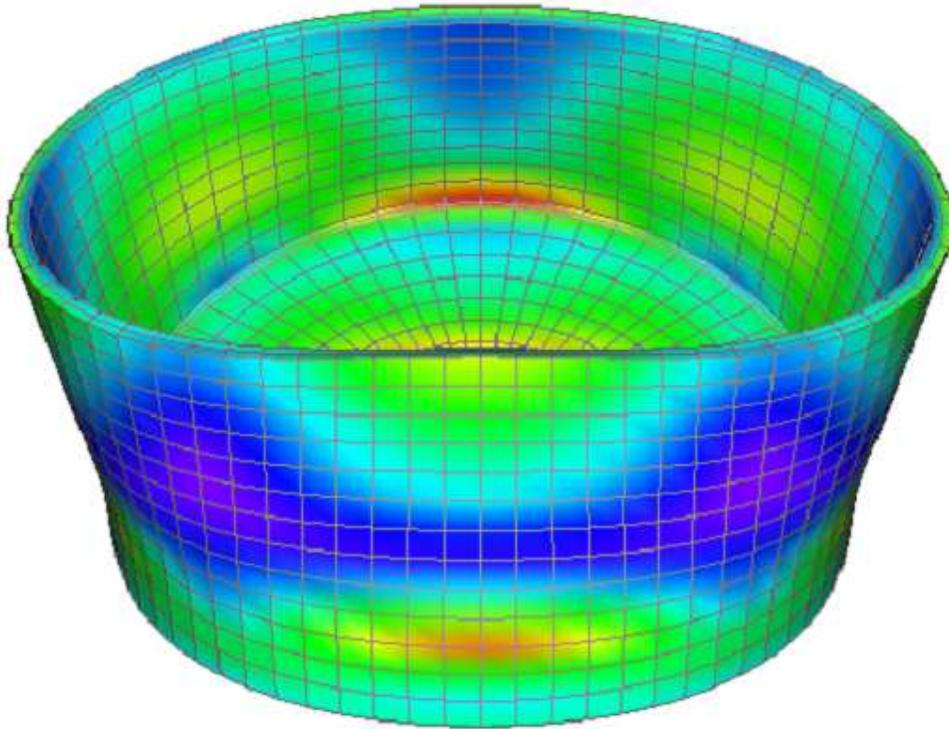
**Figure 6. Cup resonance stress pattern.**
