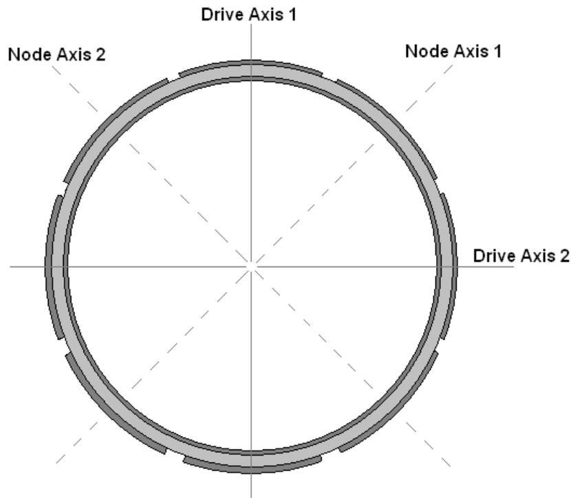
**Figure 3. Gyro electrode placement.**
