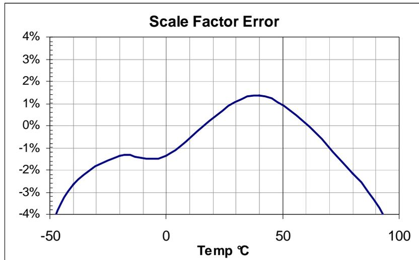
**Figure 11. Split sense electrode scale factor performance.**
