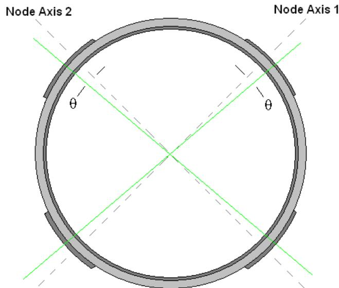
**Figure 12. Node axes with skewed electrodes.**
