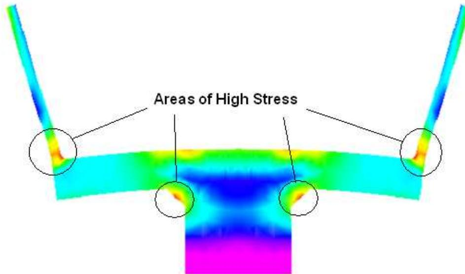
**Figure 7. Cup resonance stress pattern and displacement on the drive plane.**
