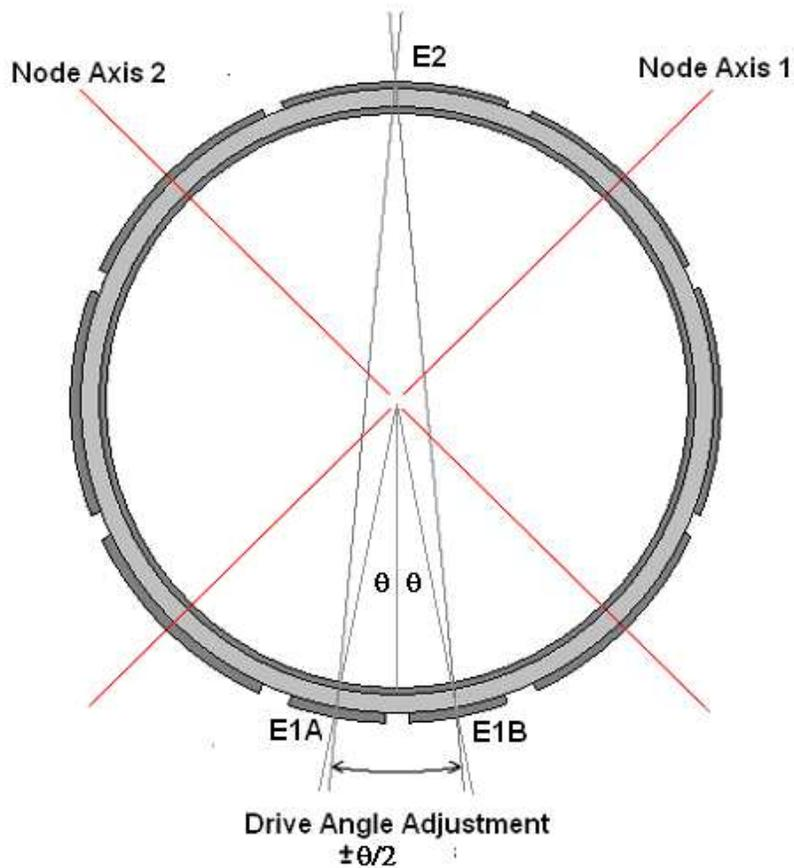
**Figure 5. Gyro split electrode geometry.**
