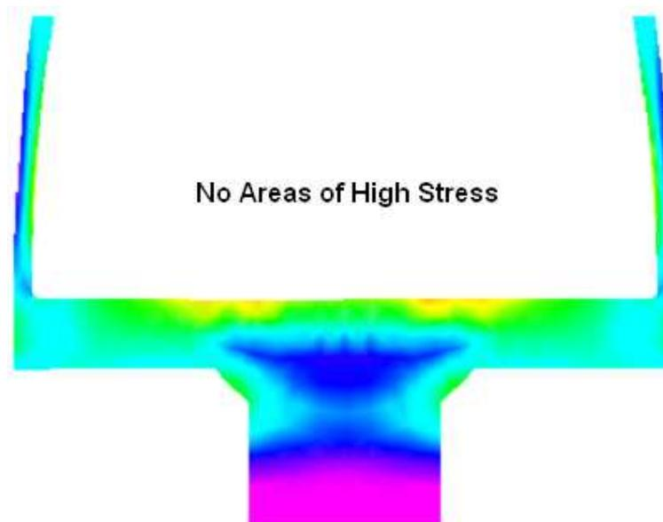
**Figure 8. Cup resonance stress pattern and displacement on the node plane.**
