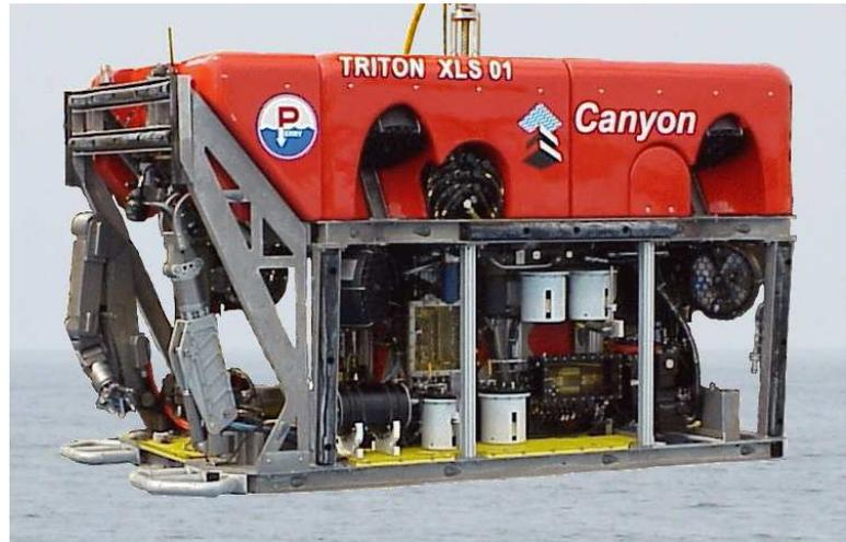
Piloting the trencher requires a full attitude sensor. Heading data is necessary to navigate the vehicle to the site. Pitch and roll data is required to assure the robot maintains a level orientation in transit and once it begins burying operations.
