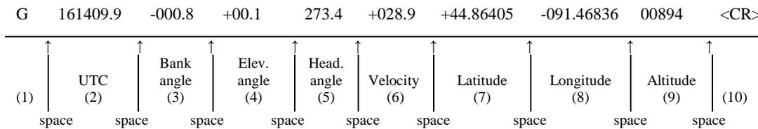
The string transmission rate can be improved by reducing the amount of information (data items) transmitted. The data items transmitted can be changed by using special commands to modify the EEPROM of the unit (see Appendix A). In addition, more channels are available for output (see Appendix A).
