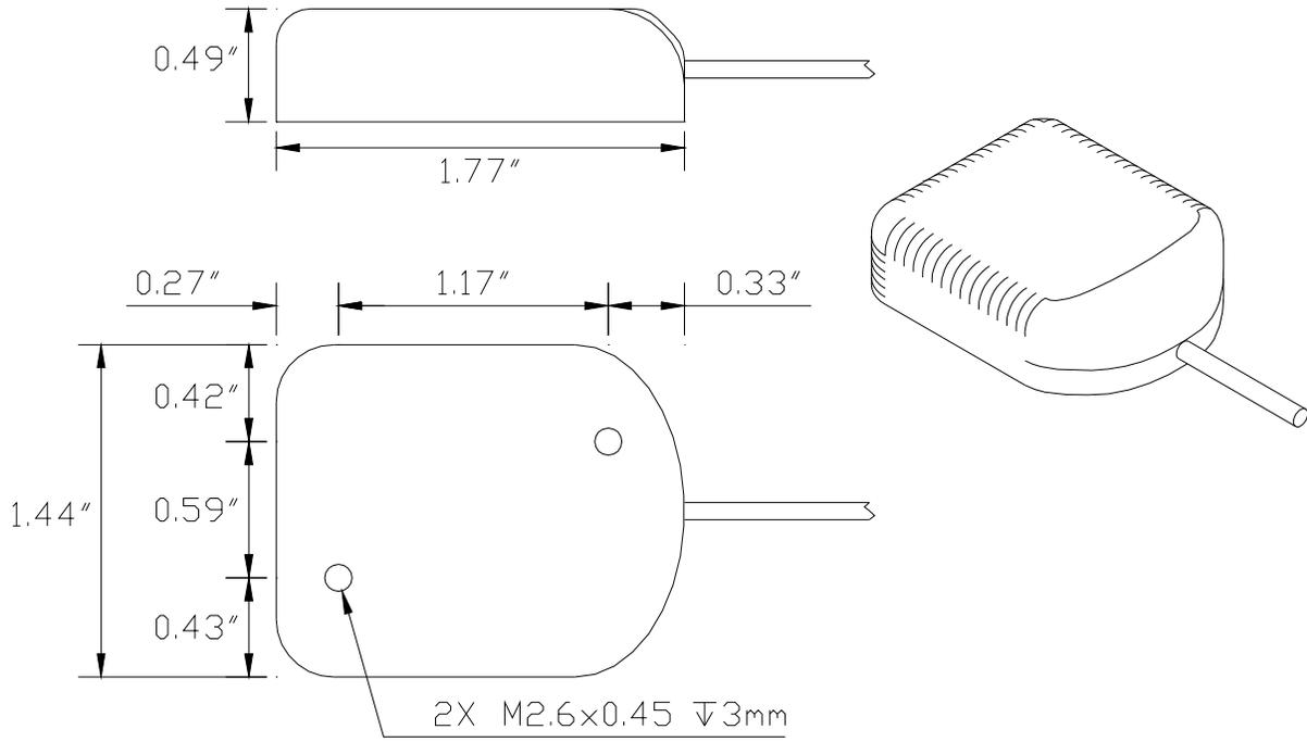
**Figure 3 Antenna Dimensions**
