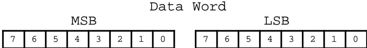
Bit 7 of the MSB is set to 1. Bits 6 to 0 of the MSB are the upper 7 bits of the data. (sign plus 6 bits of data)
