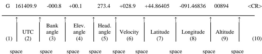
The string transmission rate can be improved by reducing the amount of information (data items) transmitted. The data items transmitted can be changed by using special commands to modify the EEPROM of the unit (see Appendix A). In addition, more channels are available for output (see Appendix A).
