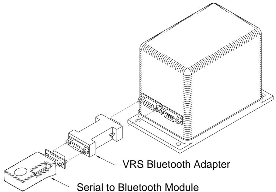
The Serial to Bluetooth Module and VRS Bluetooth Adapter are not standard features of the VRS product line, but can be obtained upon request with your order, or individually from Watson Industries.
