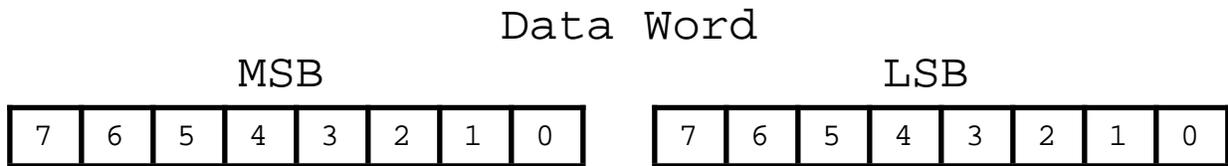
Bit 7 of the MSB is set to 1. Bits 6 to 0 of the MSB are the upper 7 bits of the data. (sign plus 6 bits of data)
