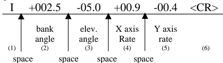
The string transmission rate can be improved by reducing the amount of information (data items) transmitted. The data items transmitted can be changed by using special commands to modify the EEPROM of the unit (see Appendix A). Additional channels are available for output (see Appendix B).
