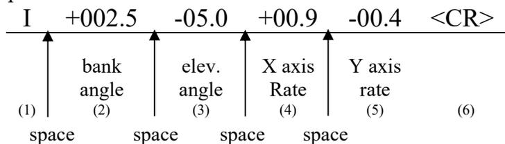
The string transmission rate can be improved by reducing the amount of information (data items) transmitted. The data items transmitted can be changed by using special commands to modify the EEPROM of the unit (see Appendix B). More channels are available for output (see Appendix A).
